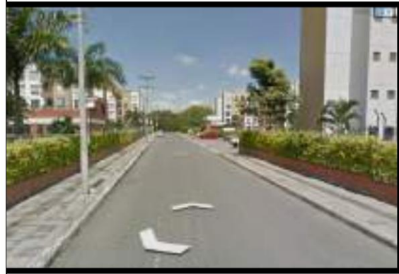
Figure 60 Sidewalks between 90 cm and 150 cm wide, with light poles in the middle Source Google Earth.
